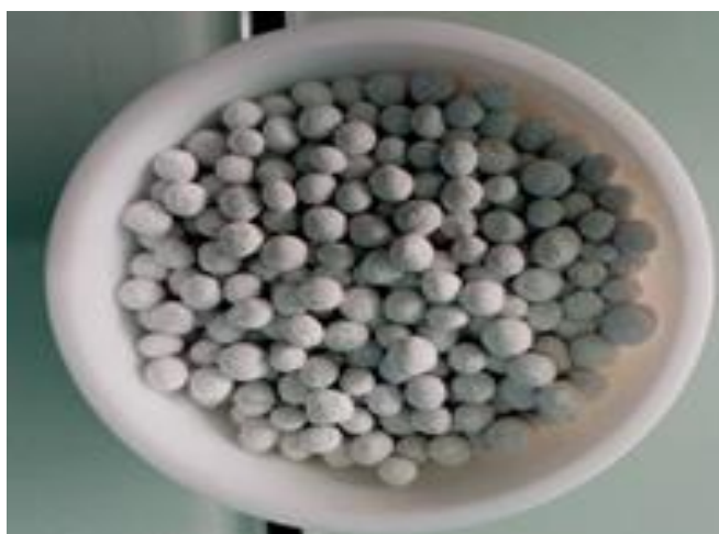
Figure 2 : Clay balls coated with \text{TiO}_2
