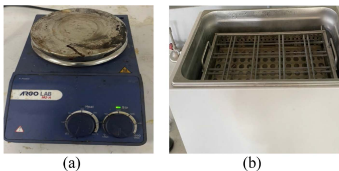
Figure 1. (a) An AGROLAB M2-A analog heating magnetic stirrer; (b) A stirring water bath.
